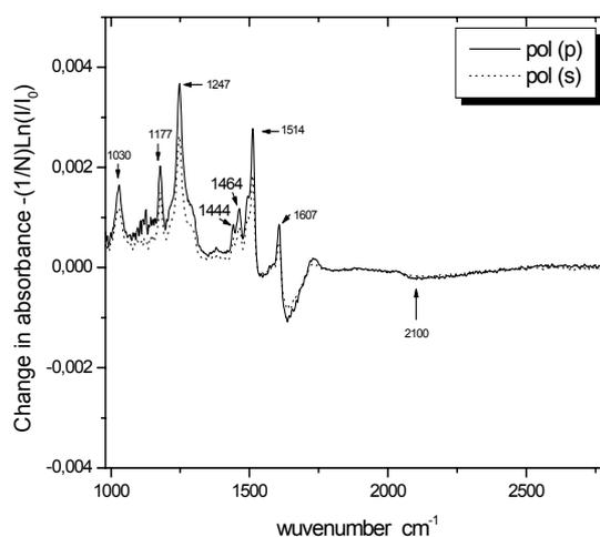
Fig. 5: IR spectrum of a silicon electrode after modification from methoxybenzenediazonium  $2\text{mM}$  in  $0.05\text{M}$  HF and  $0.05\text{M}$   $\text{H}_2\text{SO}_4$  at  $E = -0.1\text{V}$ . The reference spectrum is recorded at open circuit potential before the first cycle of grafting spectrum.
