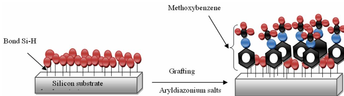
Fig. 7: Schematic representation of the modeling *grafting* of the silicon substrate by diazonium salts.
