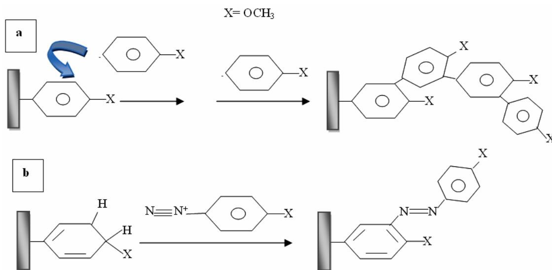
Fig. 8: Mechanism of polyphenylene multi-layers formation by aryl diazonium salt chemistry.
