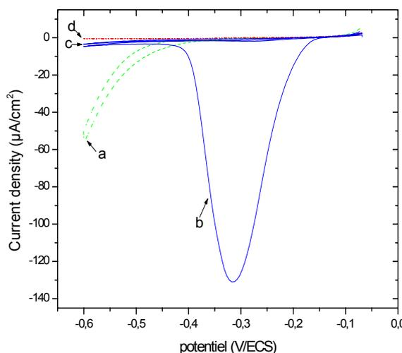
Fig. 3: Voltammograms obtained on p-Si electrode (111). (a) curve without cathode precursor and in the presence of light, (b) and (c) are respectively the first and second cycle of *grafting* in the presence of 2mM méthoxybenzènediazonium in an electrolyte composed of 0.05M HF and 0.05M  $\text{H}_2\text{SO}_4$ , (d) voltammogram in the presence of the precursor without light (no *grafting*). The scan rate is 10mV/s.
