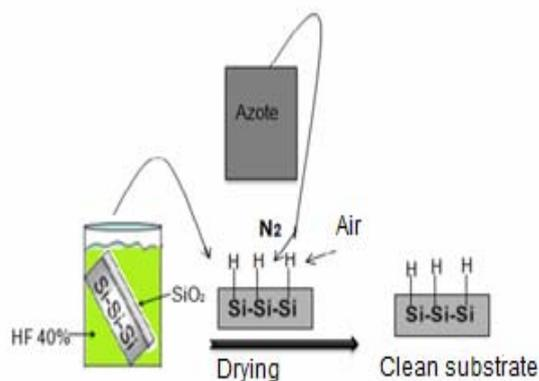
Fig. 9: Chemical treatment of silicon substrate.
