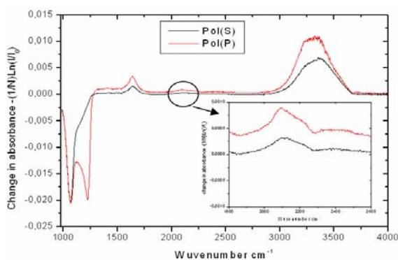
Fig. 4: In-situ IR spectrum of the hydrogenated silicon surface made the open circuit potential to  $-0.1\text{V}/\text{ECS}$  in an solution  $0.05\text{M}$  HF and  $0.05\text{M}$   $\text{H}_2\text{SO}_4$  in S polarization and P.
