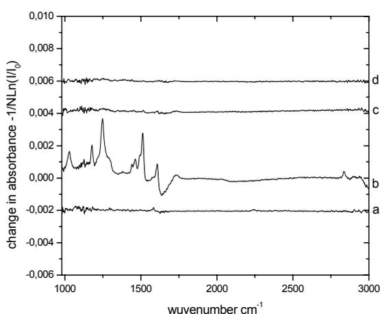
Fig. 6: In-situ IR spectrum of a silicon electrode before and after modification by methoxybenzene diazonium 2 mM in 0.05 M HF and H<sub>2</sub>SO<sub>4</sub> 0.05 M. (a) IR spectrum in an open circuit in the presence of precursor and without light - 0.1V. (b) IR spectrum open to 0.1V after the first round of *grafting* open circuit. (c) and (d) are successively 3rd and 4th cycle *grafting*.
