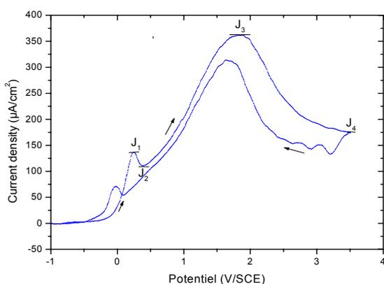
Fig. 1: Voltammogram of an electrode of the p-type silicon (111) in a solution of HF 0.05M+ H<sub>2</sub>SO<sub>4</sub> 0.05M, pH=3 and V<sub>b</sub>=10mV/s.
